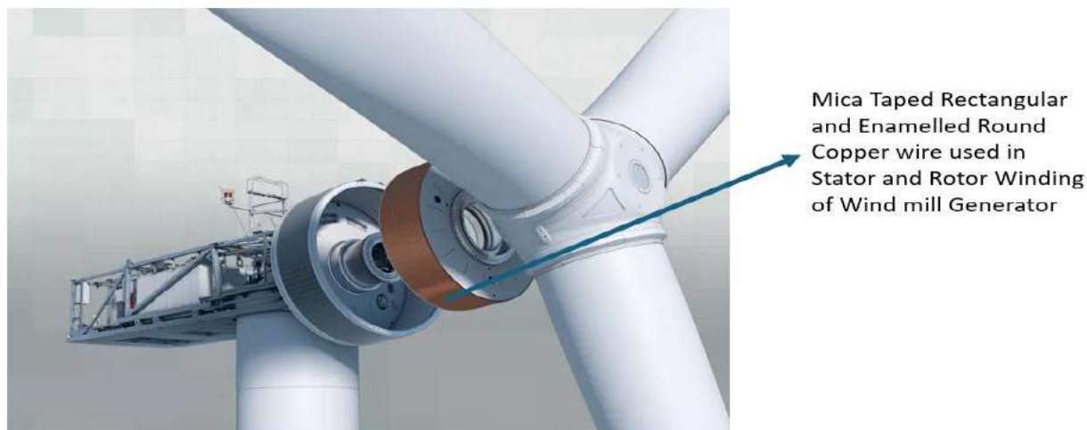
Figure 2: Use of Winding Wires in Turbine Generator
